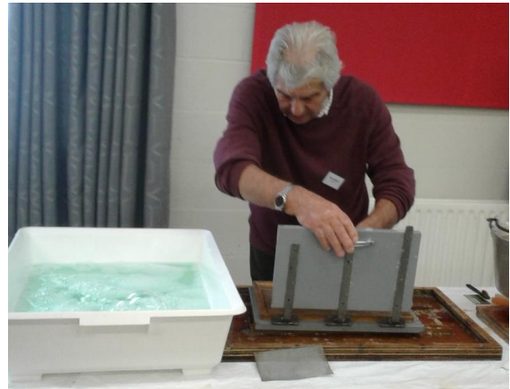
Pouring the wax into a foundation press
